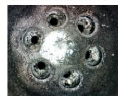
Injector nozzle after cleaning
