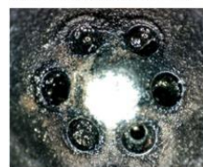
Injector nozzle before cleaning
